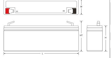
**L:** 7.00 (178) **W:** 1.37 (35) **H**: 2.36 (60) HT: 2.59 (66) Tolerances are +/- 0.04 in. (+/- 1mm) and +/- 0.08 in. (+/- 2mm) for height dimensions.
